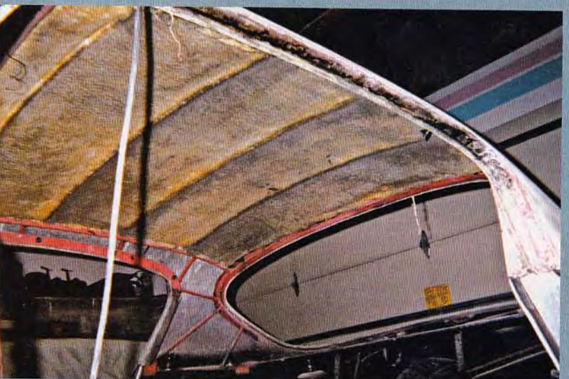
Looking toward the back window with the headliner fabric removed reveals Touring's unmistakable superleggera construction
