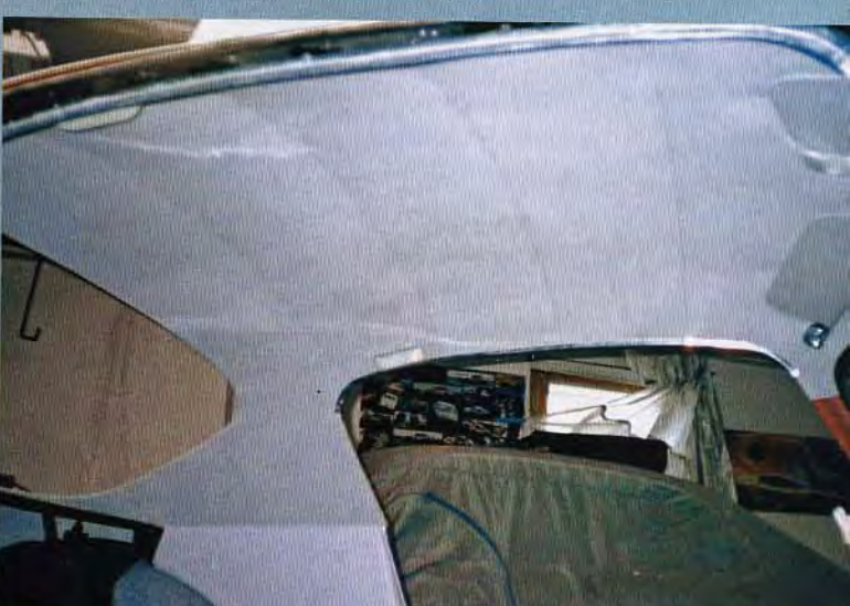
Three sleeves or darts at the front of the headliner are sewn around the roof support pipe. Edges are glued in, windows have to come out
