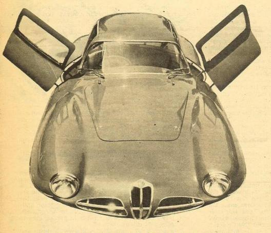
Because of the marked "tumble-home" of the body sides, the "Flying Saucer" coupe must swing its doors up at a sharp angle. Side view (next page) shows exhausts along side.
