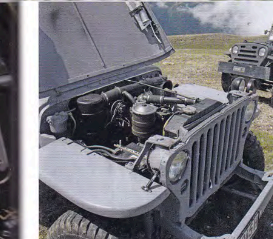
Left to right: torquey 'Go-Devil' sidevalve offers the most punch here; cutaway sides made it easy for GIs to hop in and out; Willys cabin has been superbly restored
