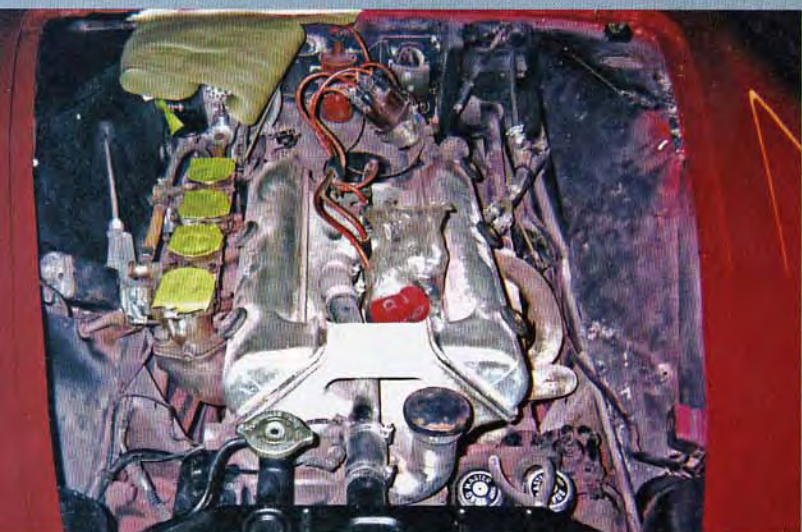
Inner fenders are now covered with quilting, so overspray wasn't an issue. Small panel in the wheel well gives access to belts and hoses
