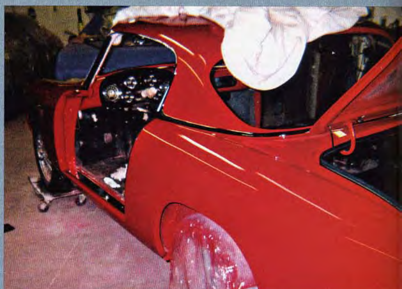
Paint was razor-stripped off and Touring's primer left on in most places; Chromalite body filler used on the uneven aluminum body shell
