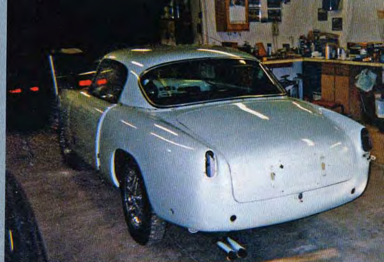
Next was to remove the glass, upholstery and interior. Restorer decided not to remove the complicated dash, loosened it enough for cleaning
