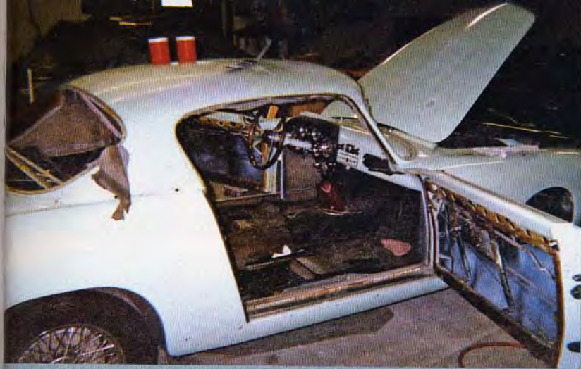
Careful removal, evaluation and storage of exterior trim is a vital first step. Everything was there, aluminum and chrome refinished
